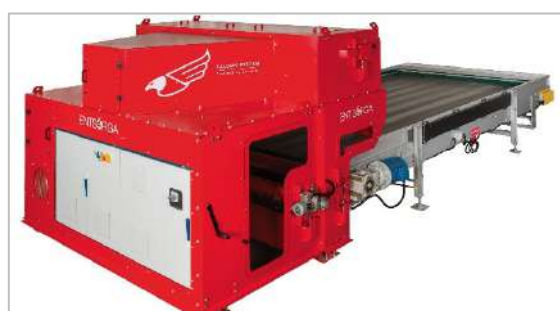
(2) NIR SEPARATOR FALCON™ TO REMOVE CHLORIBNATED PLASTICS
